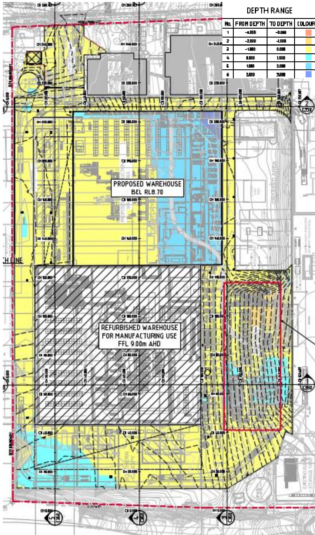
Figure 4 – Cut and Fill Plan Indicating Extent of Excavation
