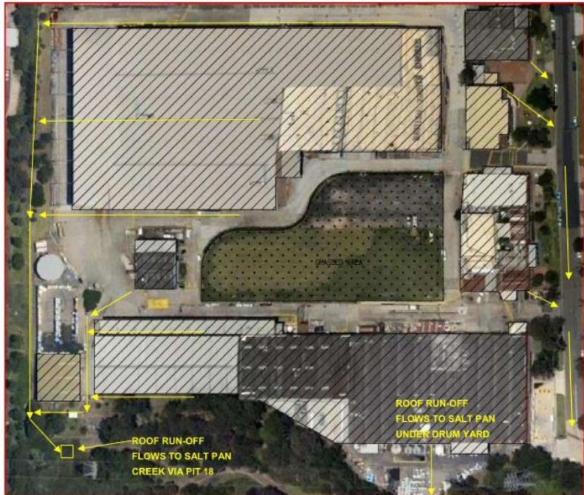
Figure 22. Existing Roof Areas Stormwater System (Source: Costin Roe, 2024)
